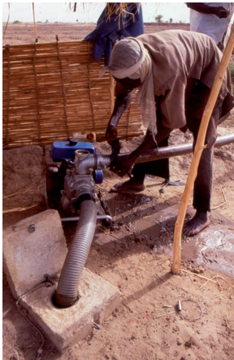
Figure 1. Small scale irrigation from river floodplains in Northern Nigeria using suction pumps.
