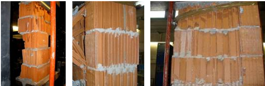
Figure 2.9 Typical failure modes of clay masonry under compression.
