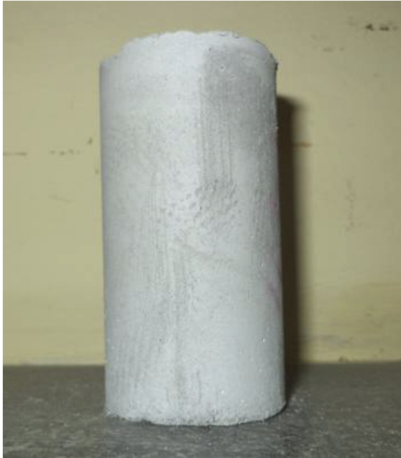
Figure 15.3 Geopolymer mortar cylinders.
