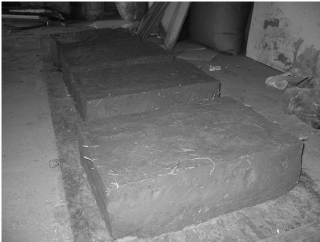
Figure 16.3 A typical prismatic adobe block.
