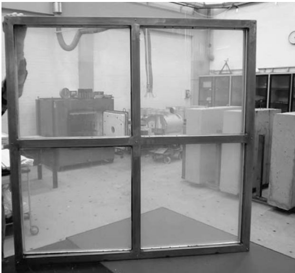
10.4 An aerogel window manufactured by joining four optimized aerogel tile prototypes in a test frame (Jensen et al. , 2004).
