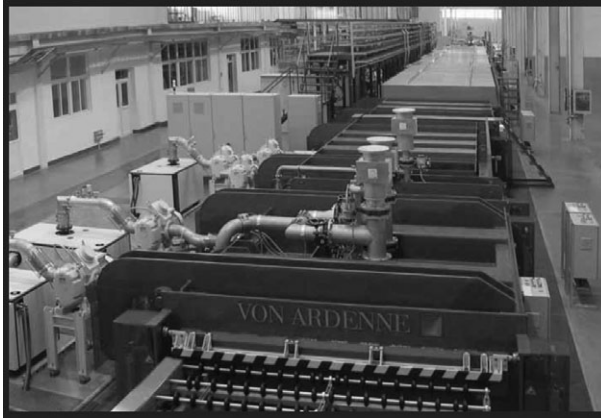
8.16 Photograph of a manufacturing plant for making multilayer coatings on full-size glass panes.
