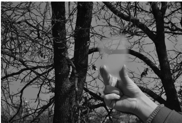
10.3 View through a monolithic aerogel sample (sample supplied by AIRGLASS, Sweden, 2010) (Buratti and Moretti, 2012b).
