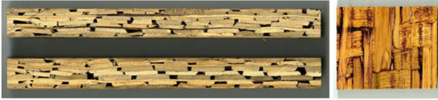
Fig. 10.34 Different forms of ply bamboo panels used as container boards (Schülke 2009)
