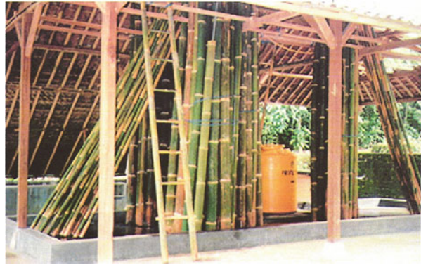
Fig. 9.28 The Vertical Soak and Diffusion method for treating bamboo culms at the Environmental Bamboo Foundation in Ubud, Bali (Liese and Kumar 2003)
