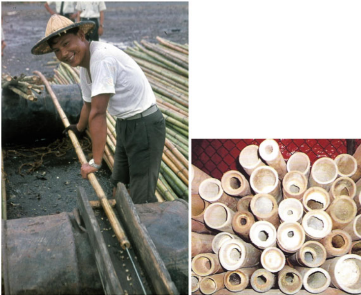
Fig. 9.31 Ruptured nodal walls by a long iron stick to ease penetration in Thailand (Liese and Kumar 2003)
