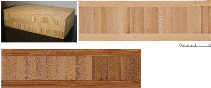
Fig. 10.35 Ply bamboo based on splits, bleached or natural color, and darkened by heat treatment (Waitkus)
