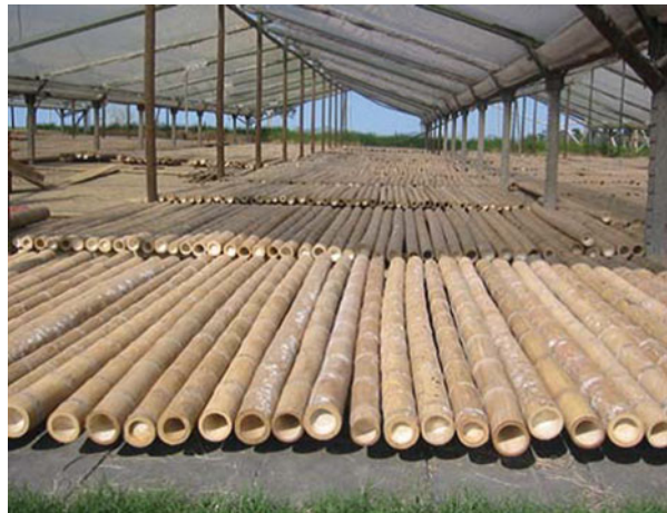
Fig. 9.32 Horizontal stacking bamboo culms for air-drying under cover (Montoya-Arango 2006)
