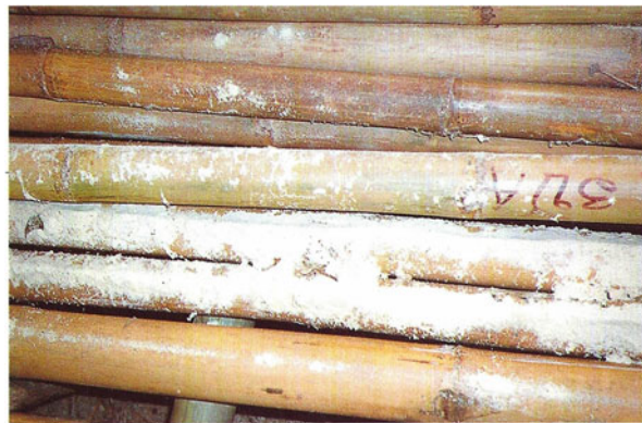
Fig. 9.6 Powdery mass of pellets due to beetle attack (Liese and Kumar 2003)
