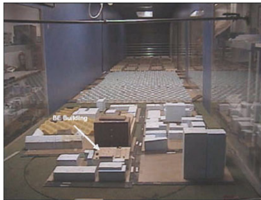
Figure 11. Typical wind tunnel set-up for a pedestrian wind assessment study.
