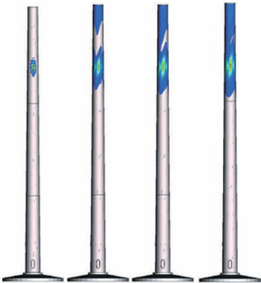
Figure 23. 1 st buckling eigenmode – Perfect shell and fabrication classes A, B, C dimple imperfect shells (perfect shell & fabrication classes A,B,C)
