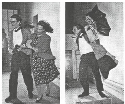
Figure 8. Wind tunnel exposure of people at 70 km/h winds.
