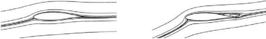
Figure 6. Streamlines for the same airfoil at two different angles of attack: \alpha = 5 deg attached airflow on the left, \alpha = 15 deg separated flow on the right. Cfr. Hansen (2008)
