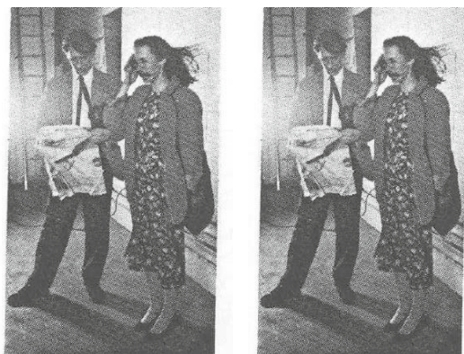
Figure 7. Wind tunnel exposure of people at 20 (left) and 40 (right) km/h winds.
