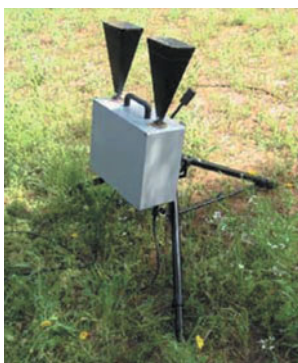
Figure 49. Prototype of the interferometric sensor.
