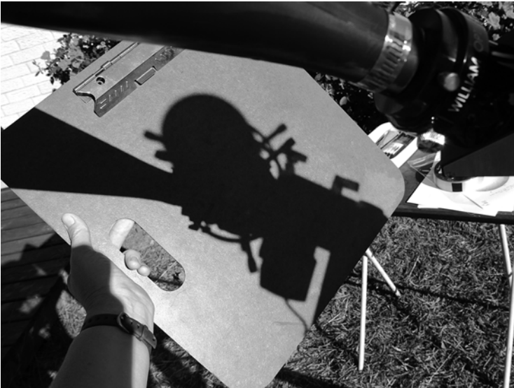
Fig. 1.25 Lengthened shadows indicate that the telescope is not in alignment to the Sun. (By Erika Rix)
