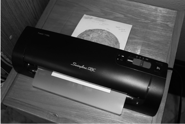
Fig. 1.44 Laminating machines use heat to permanently seal sketches between thin layers of plastic. (By Erika Rix)
