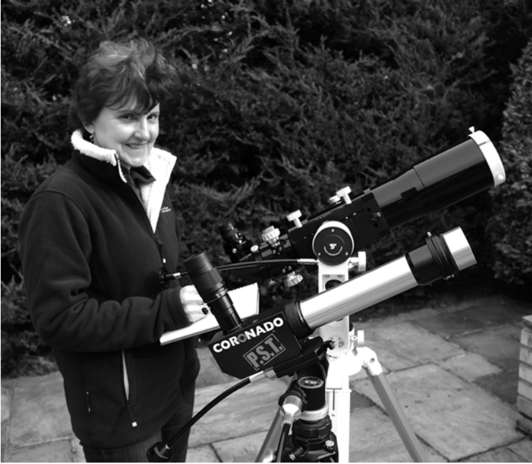
Fig. 1 Sally Russell with her Coronado double-stacked PST and Astro-Physics 105 mm f/5.8 Traveler fitted with a Kendrick white light filter
