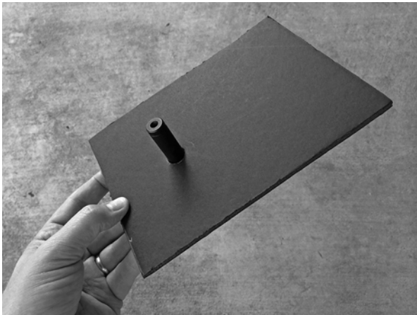
Fig. 11.14 The pocket spectroscope is fitted with a homemade sun shield to improve contrast and protect the children's eyes from direct sunlight. (By Erika Rix)
