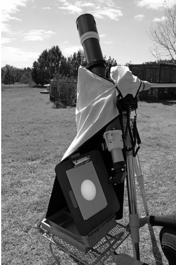
Fig. 4.26 Solar eyepiece projection using a 102 mm f/9.8 refractor with a 12 mm eyepiece and a tracking mount. The telescope's aperture was stopped down to 51 mm, 12 mm eyepiece. (By Erika Rix)
