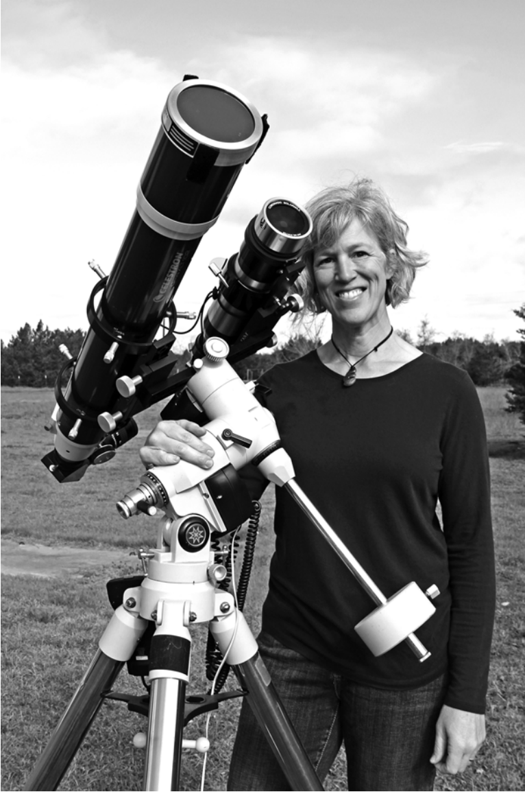
Fig. 4 Erika Rix with her internally double-tacked H-alpha Coronado Maxscope 60mm and a Celestron Omni XLT 102 mm f/9.8 refractor fitted with a Thousand Oaks type 2+ glass solar filter, optical density 5.0
