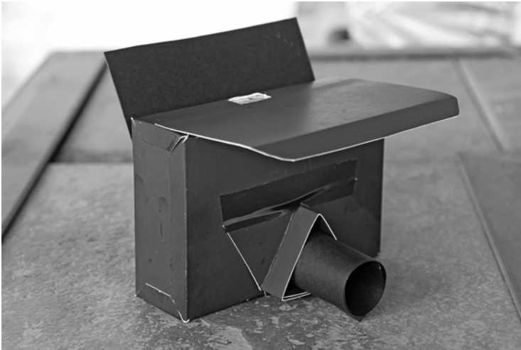
Fig. 11.15 Homemade spectroscope using cardstock, black paper, electrical tape, glue, an aluminum can, and a DVD. (By Erika Rix)
