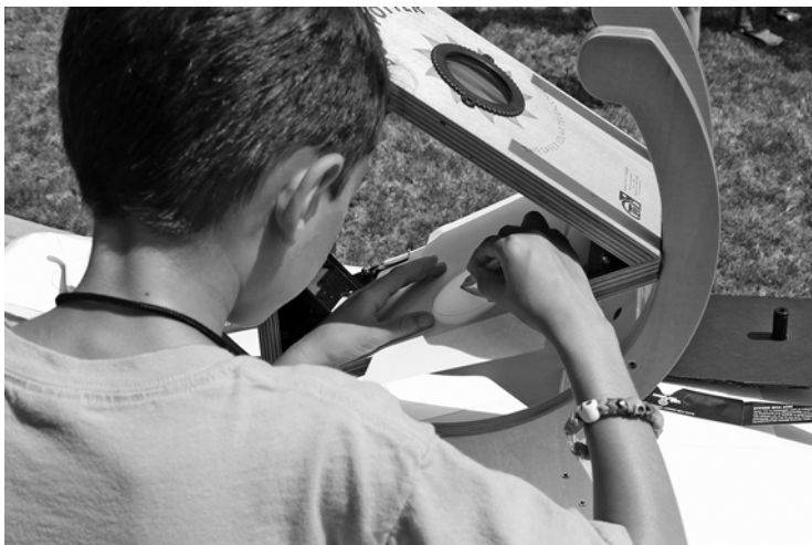
Fig. 11.7 The sunspots can either be traced onto the projected image or drawn on a separate sheet of paper next to the telescope. (Courtesy of Tara Krzywonski, Texas, USA)
