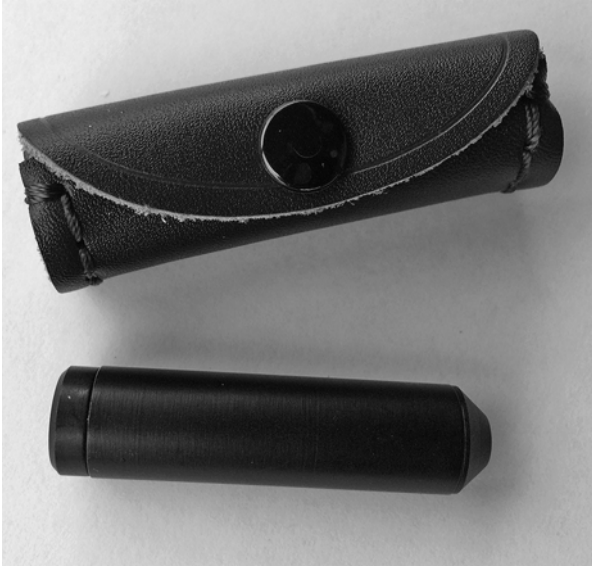
Fig. 11.13 An inexpensive, entry-level pocket spectroscope that is perfect for outreach. (By Erika Rix)
