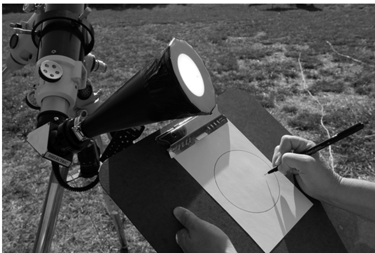
Fig. 4.14 Hold the sketch close to the Sun Funnel to easily cross-reference between the two views. (By Erika Rix)
