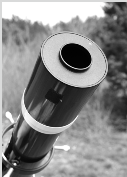
Fig. 4.25 When the center of a dust cover is removed, it can serve as an aperture mask. (By Erika Rix)
