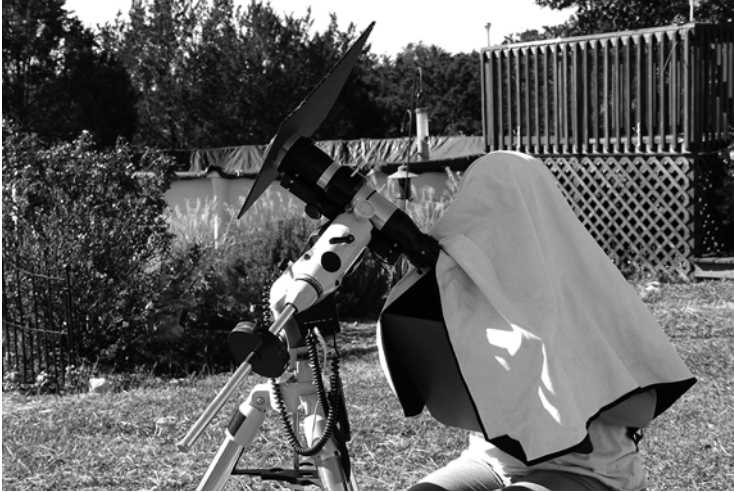
Fig. 1.12 Combining the use of a solar cloth with a sun shield preserves dark adaptation for sketching the faintest prominences. The sketch board is easily placed under the cloth with enough ambient light to sketch by. (By Erika Rix)
