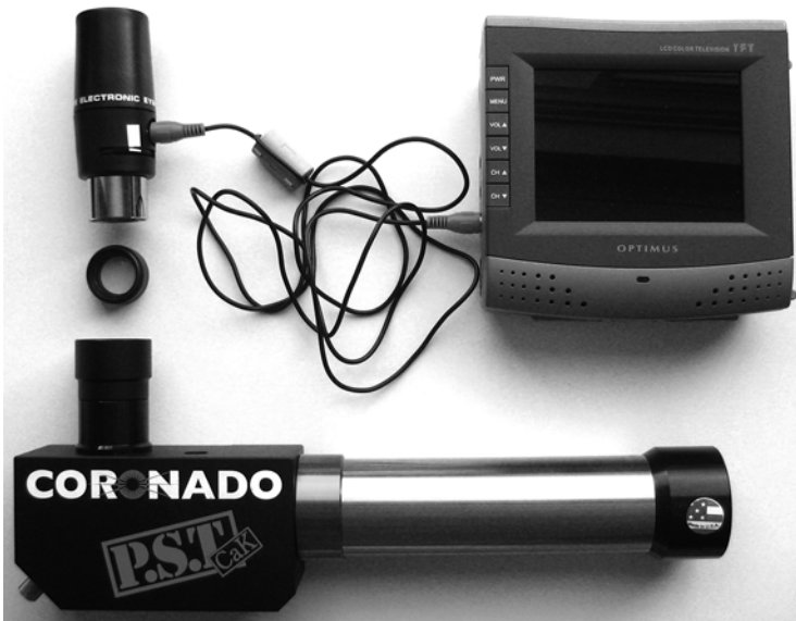
Fig. 6.10 Clockwise from upper left : electronic eyepiece, video output cable, 5-in. portable LCD TV, Coronado CaK PST, \times 1.6 supplementary lens. (By Sally Russell)
