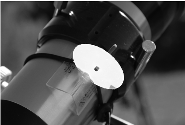
Fig. 1.28 Minimal or no shadow on the Helio-Pod Solar finder indicates alignment to the Sun. (By Erika Rix)
