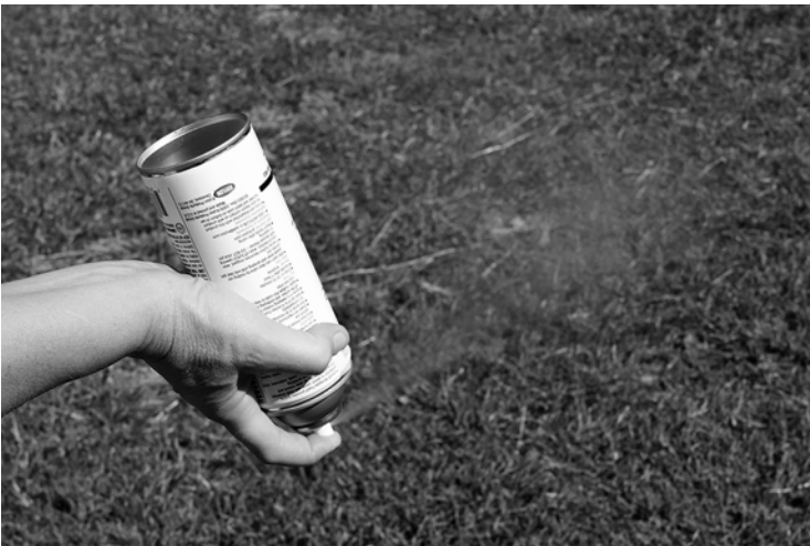
Fig. 1.43 Turn the can upside down and spray to clear the nozzle. (By Erika Rix)
