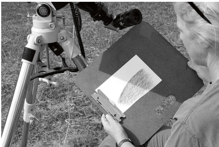
Fig. 1.22 Demonstrating the effectiveness of a sun shield. The right side of the sketch is shaded underneath the shield. The left side of the sketch remains within the glare of direct sunlight. (By Erika Rix)
