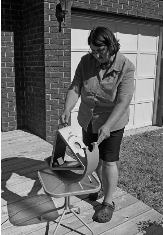
Fig. 4.2 Kim Hay is seen aligning the Sunspotter with the Sun's path. (By Kim Hay)
