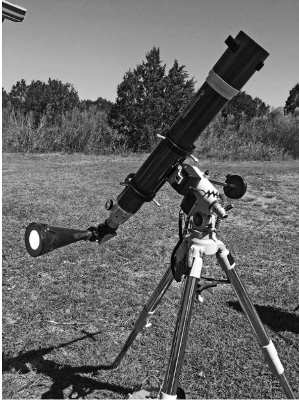
Fig. 4.12 Sun Funnel attached to a 102 mm f/9.8 refractor on a driven mount. (By Erika Rix)
