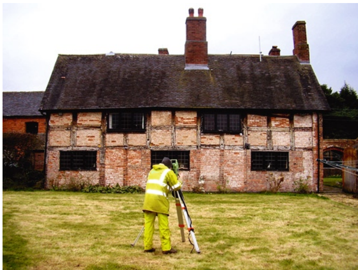
Fig. 6.4 Historic building recording in action, using electronic distance measuring equipment on a site in Staffordshire. Photograph by Sophie Watson, Clwyd-Powys Archaeological Trust
