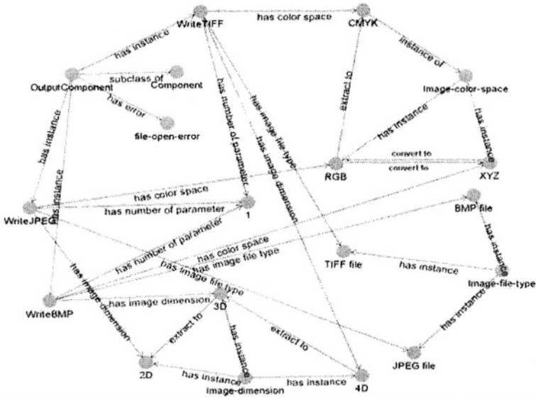
Figure 3. A part of the knowledge base (implemented in the CREEK system) for components in the image processing field.
