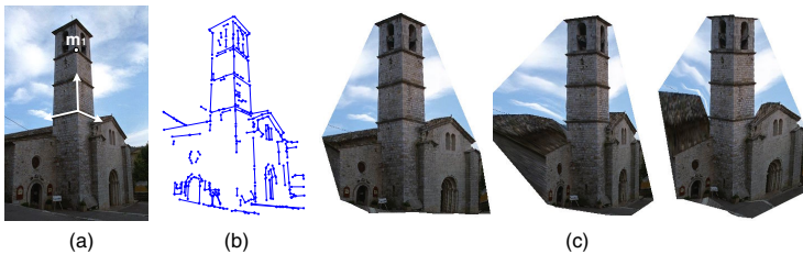
Fig. 3. (a) One of the two images of Valbonne church; (b) the detected line segments; (c) the reconstructed model under different viewpoints with texture mapping
