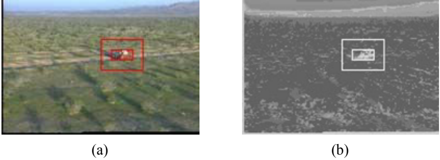
Fig. 1. Illustration of center-surround approach. (a) the original image. (b) corresponding weight map.
