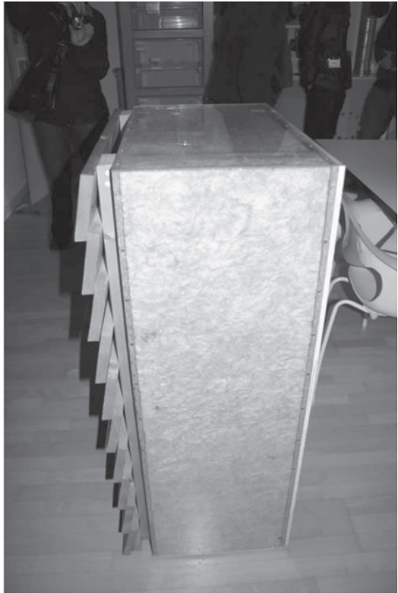
Figure 5.7 Section of the external wall showing the thickness of the thermal insulation
