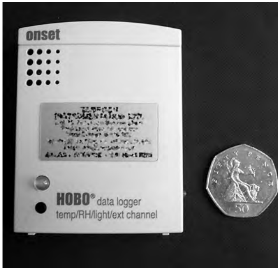
Figure 9.1 Example of a portable data logger used for measuring temperature and relative humidity
