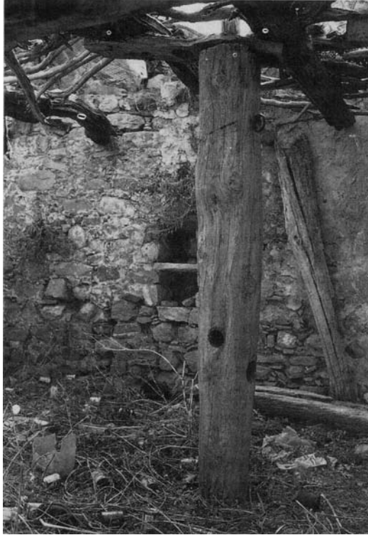
Figure 2.12. Botzargati (windlass) in olive press house in Monastiraki.
