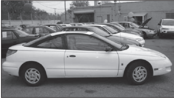
Figure 9 Door panel made of filled PC/ABS; fenders and quarter panels made of Noryl GTX.
