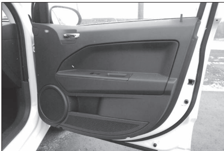
Figure 6 Door module made of TPO.
