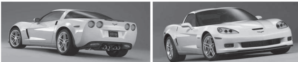
Figure 11 RIM fenders in the C6 GMX 245 Corvette.
