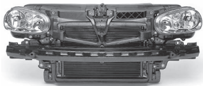
Figure 13 Assembled prototype for testing at Volkswagen.
