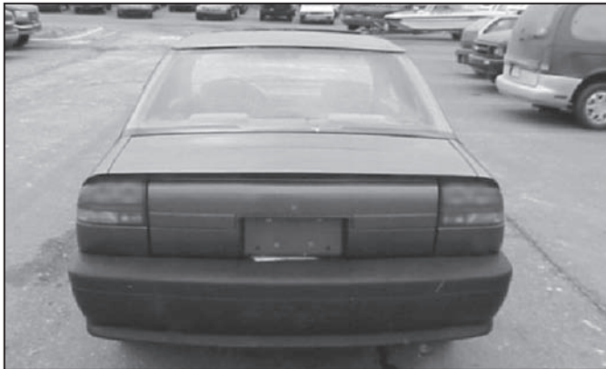
Figure 10 Rear panel made of filled PC/ABS.
