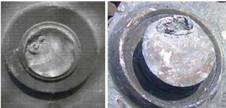
Fig. 7.40 Concave and convex surfaces in an axle in a railway failure
