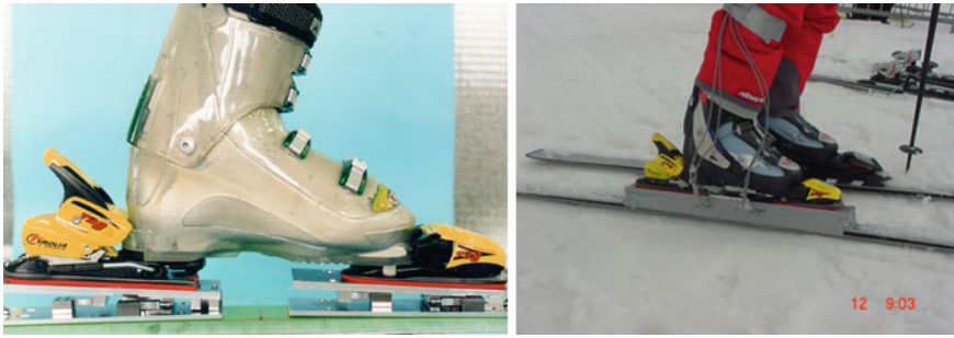
Fig. 7.3 Device to measure the six forces and moments transmitted by a ski boot to a ski
