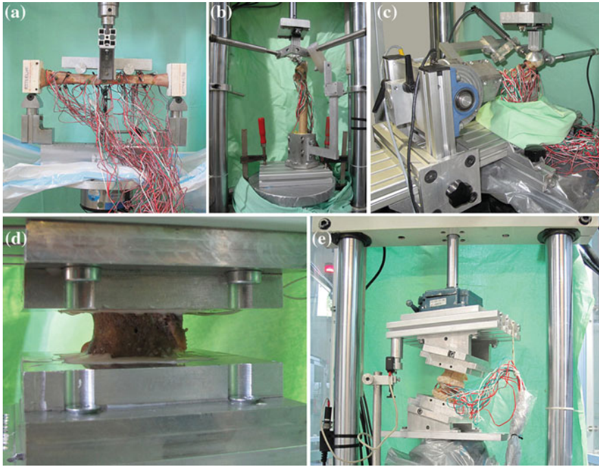
Fig. 10.4 Examples of in vitro biomechanical experiments to measure the stiffness, strain distribution and strength of intact and operated bone segments: a four-point-bending of a human tibia; b single-leg-stance loading of a femur implanted with a hip stem; c sideways fall simulation on a human femur; d compressive testing of an isolated vertebra and e compression-bending of a three-vertebrae spinal segment. The strain gages that were used for measuring strain on the bone surface are visible (Copyright of the VPHOP consortium; reproduced with permission)
