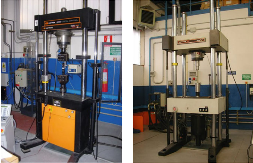
Fig. 8.1 Example of universal testing machines of 250 and 500 kN capacity (INSTRON Ltd.)
