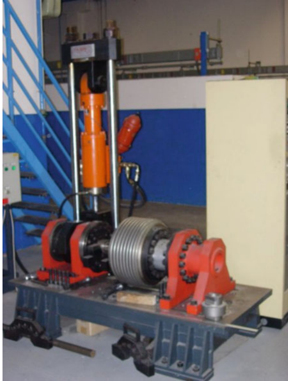
Fig. 8.18 Self-manufactured testing apparatus built for alternate torsion testing with loading capacity up to \pm 25 \text{ kN m}
