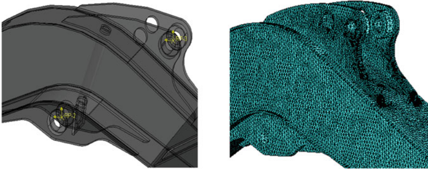
Fig. 1.2 The forward numerical model as a reference model for experimental measurements. The finite elements method reduces complex structures to a numerous series of simple elements for which the system matrix is assembled. See a case study in Sect. 7.10.1 in Chap. 7
