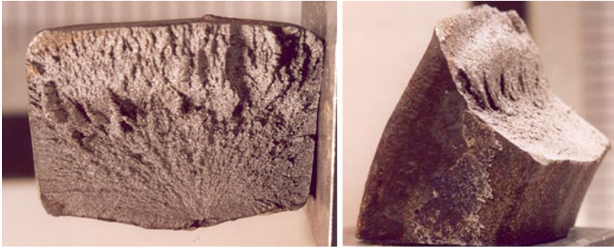
Fig. 7.38 Failure surface of a curved bar. The enucleation point, the propagation area and the final brittle failure area at 45^\circ can be detected
