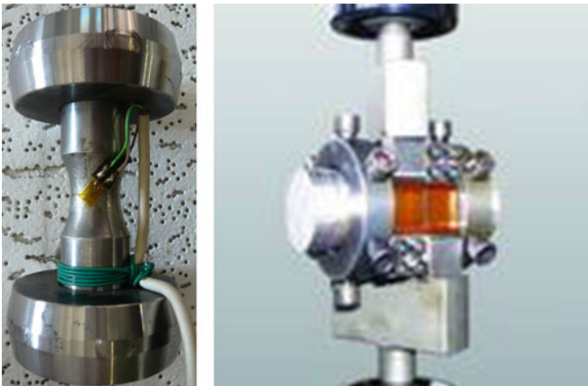
Fig. 7.9 Instrumented test specimen for alternate torsion and related equipment to be mounted on a vibrofore [26]
