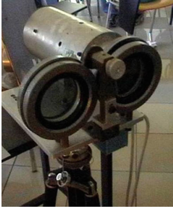
Fig. 3.39 Self-manufactured reflexion polariscope
