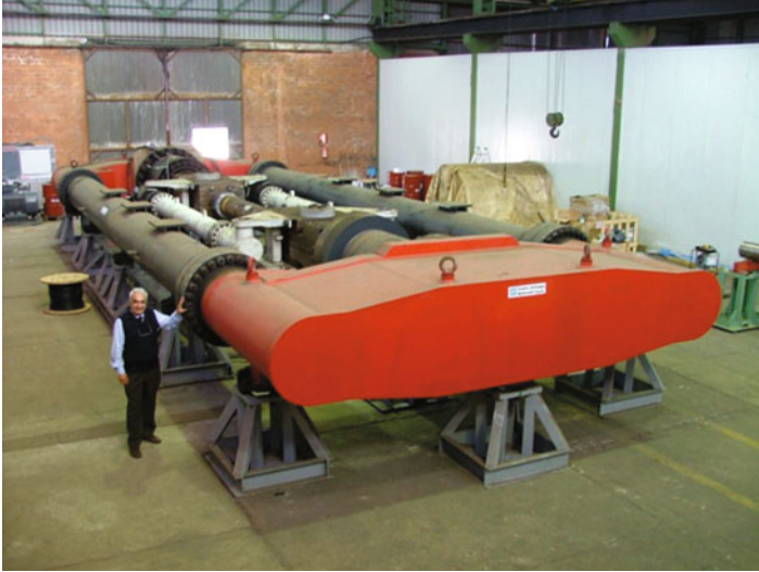
Fig. 6.29 Static test equipment for pipes and joints of 25 MN capacity (manufacturer: Giuliani-Forlì, Italy)
