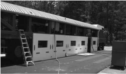
Figure 1. Insulated panels used for temperature control.
