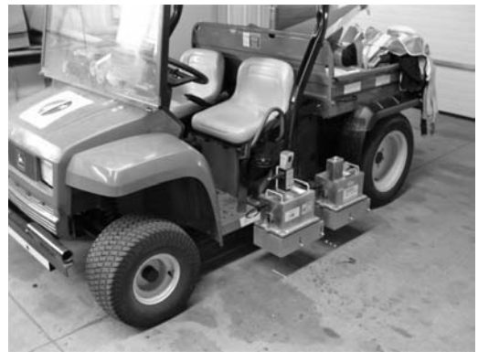
Figure 11. Lightweight profiler for measuring IRI and RN.
