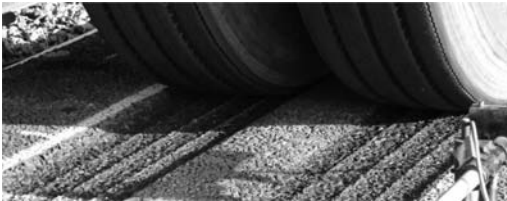
Figure 2. HVS dual tires in channelized mode on a test pavement.
