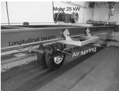
Figure 1. Components of the test track (longitudinal direction).
