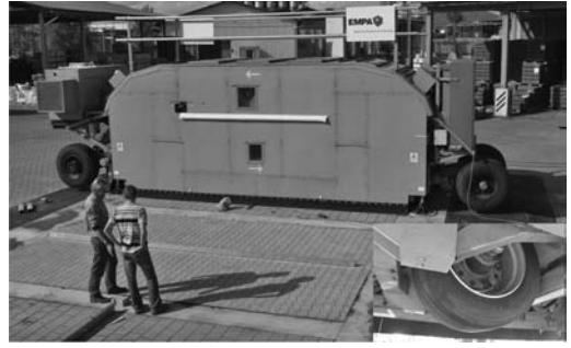
Figure 5. Mobile Load Simulator MLS10 with super single tires.
