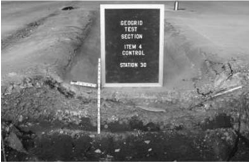
(b) Control section with 2" AC after 24,000 ESAL
