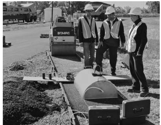
Figure 9. Portable flux chamber for measuring emissions during paving.
