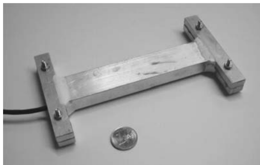
Figure 5. Asphalt strain gauge with cover (Rabe, 2004).
