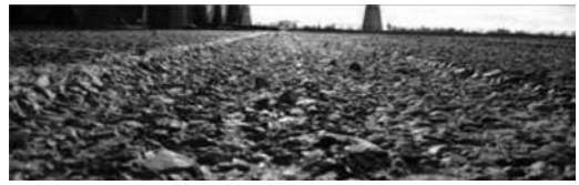
Figure 7. Horizontal view of the wheelpath after HVS testing.
