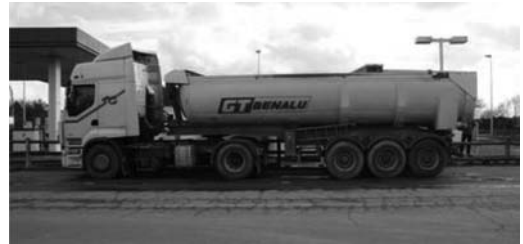
Figure 18. 44 ton heavy vehicle with tridem rear axle system, wheelbase = 112 cm.
