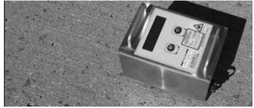
Figure 3. Ames Engineering Laser Texture Scanner used to measure pavement surface texture.
