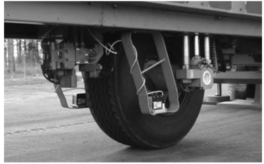
Figure 2. Laser profiling system for rut depth measurement.
