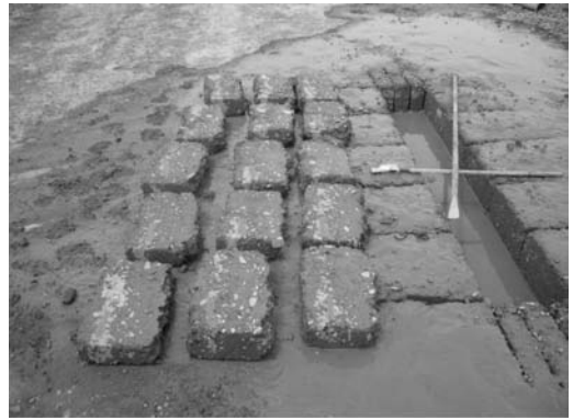
Figure 13. Cemented material slabs extracted from the field trial.
