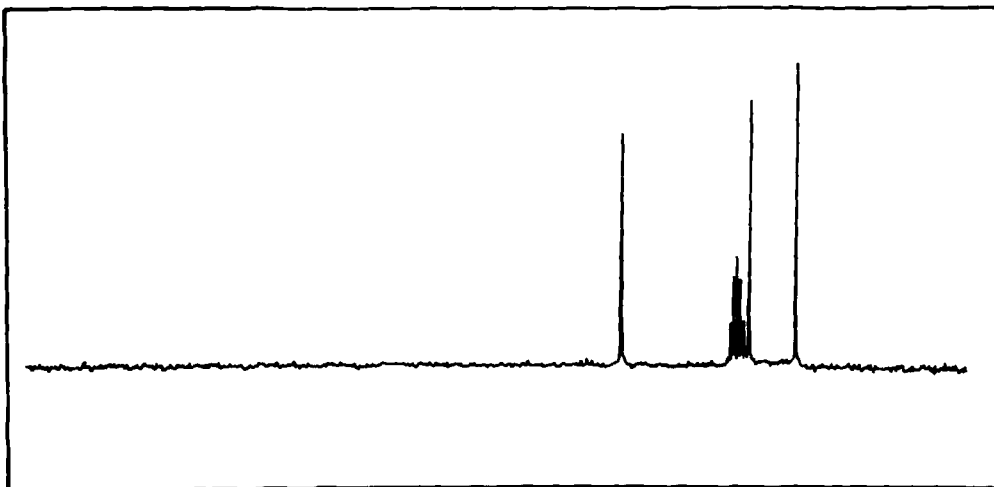
Figure 3 : Proton-decoupled carbon-13 nuclear magnetic resonance spectrum of Busulphan in DMSO-d 6 using TMS as reference standard.
