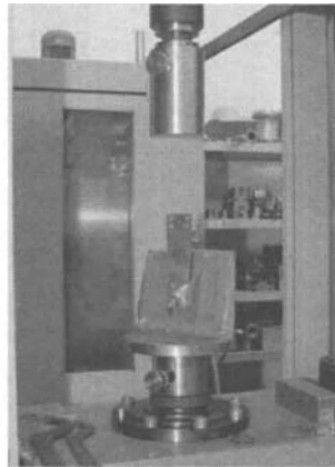
Figure 20: Load introduction test set-up
