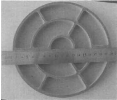
(a) \phi 110 green samples before machining
