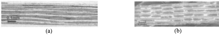
Figure 7. Optical micrographs of fiber preforms (a) before impregnation by the mineral powders and (b) after impregnation. Silicon nitride + sintering aid powders correspond to white contrast between the tows (b).
