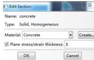
Fig. 7.15 Choosing the concrete material. Abaqus® screenshot reprinted with permission from Dassault Systèmes.
