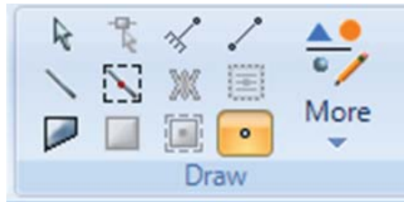
Fig. 9.12 Selecting frame elements from draw module. SAP2000 screenshot reprinted with permission of CSI.
