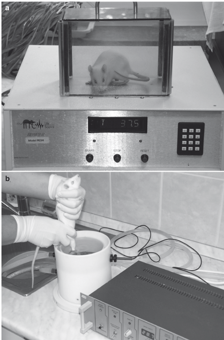
Fig. 1. The increasing-temperature hot plate (Panel a) and the increasing-temperature water bath equipment (Panel b)
