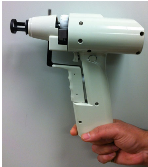
Fig. 1 Helios gene gun with a cartridge holder and a nosepiece in place. The diffuser is placed in the back of nosepiece (Image provided by Dr. Suneet Mehrotra)
