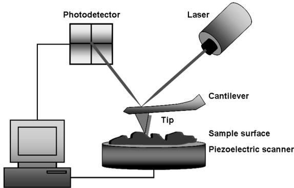
**Figure 9.1** Drawing of the basic principle of an atomic force microscope. A cantilever bearing a very small tip (probe) moves along the sample surface attached to a piezoelectric scanner. The tip experiences attractive or repulsive forces. A laser and a photodiode are used to measure these forces.
