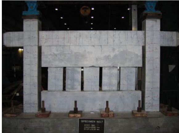
Fig. 3.3 “Ductile shear wall” with multiple SHCC dampers
