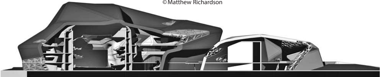
Longitudinal section through the Opera House (left) and the multipurpose hall (right)
