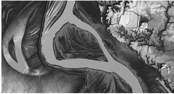
FIGURE 6.11 Five-m DEM derived from lidar data of Profit Island in the Mississippi River Basin. (Courtesy of 3001 Spatial Data Corporation.) (See color version on accompanying CD.)
