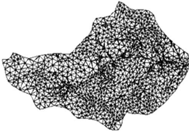
FIGURE 6.6 Example of topographic map derived from a TIN.
