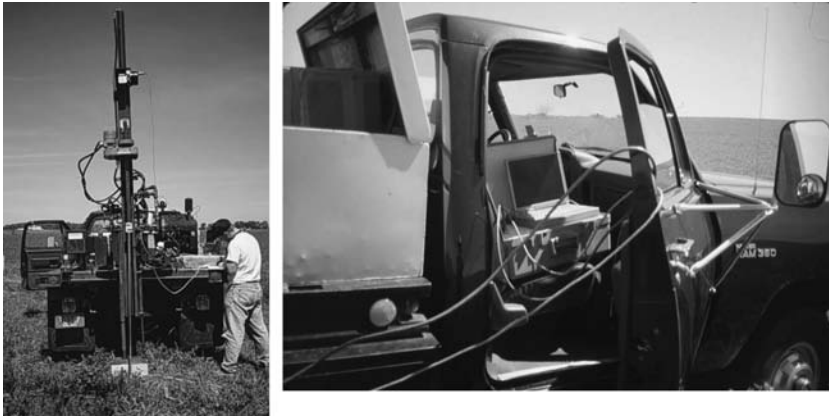
FIGURE 5.3 Truck-mounted PCP system. (Courtesy of Soil Science Department, University of Wisconsin, Madison.)
