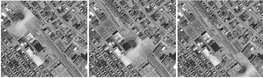
Figure 23.2 A sequence of vehicular noise representation with a peak of approximately 85 dbA. Taken from an animation of a motorcycle on Newport Ave., Quincy, MA.
