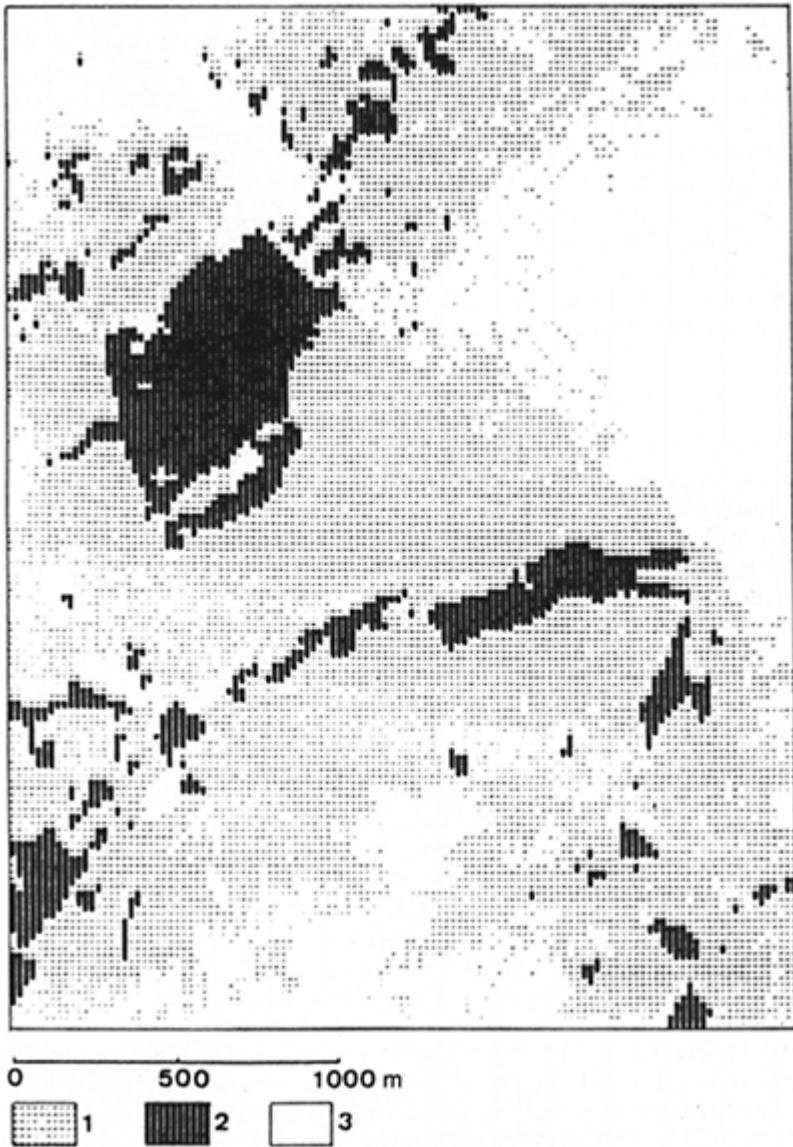
Figure 10.6. Visibility range of woodland in the Hoegaarden study area calculated on the combination of a classification and a digital relief model (1) Visibility area of woodland; (2) woodland; (3) woodland not visible.
