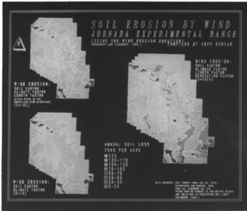
Figure 2.4. Vector GIS coverages of wind-erosion rates for a portion of the Jornada Desert, estimated using the US Department of Agriculture wind erosion equation and GIS overlay of environmental data. The three maps are of coverages generated using different combinations of environmental data.
