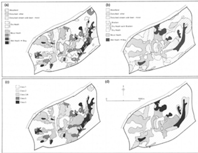
Figure 15.2. (a) Vegetation composition classification based on detailed field survey and air photograph interpretation, (b) Vegetation composition classification for the same area as map (a) based on interpretation of a false-colour composite derived from 20 and 10m resolution SPOT HRV data, (c) Winter rainfall acceptance potential map derived from the vegetation classification presented in (a), (d) Winter rainfall acceptance potential map derived from the vegetation composition classification presented in (b).
