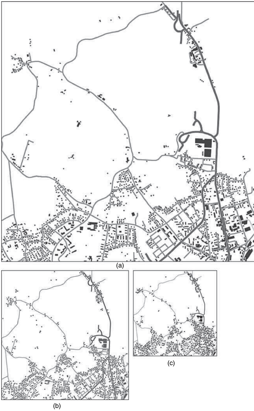
Figure 6.7 Automatic generation of different target scales from cadastral building data: 1:25 000 (a); 1:50 000 (b); 1:75 000 (c)
