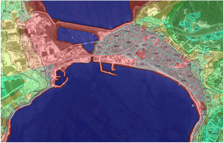
Fig. 2. Areas of a certain run-up risk for Tsunamis overlaid with land-use data and population density of residential areas (Kemper et al. 2005)
