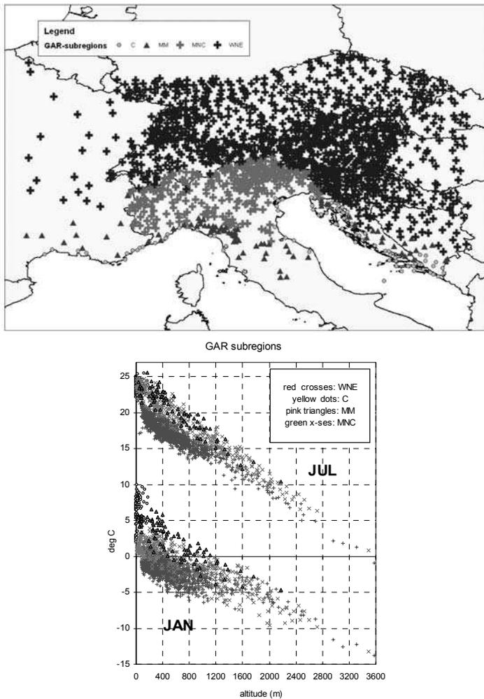
**Figure 15.5.** Relation between air temperature and altitude for individual sub-regions (bottom). The sub-regions (top) were derived from the residual maps shown in Figure 15.4
