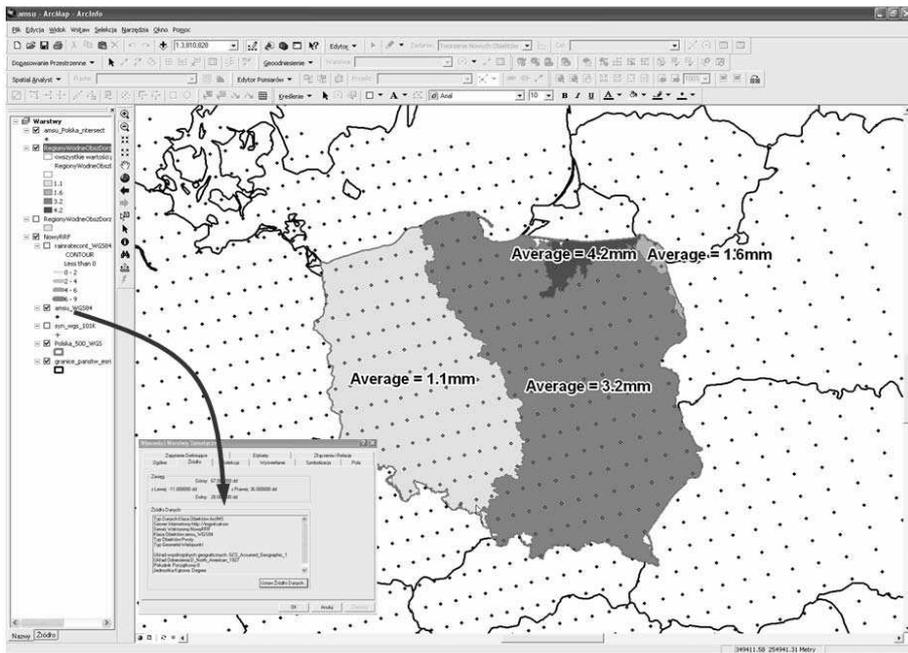
**Figure 3.4.** Average precipitation in Polish catchment areas, assessed on the basis of satellite image interpretation: example using WFS as a data source for further analyses
