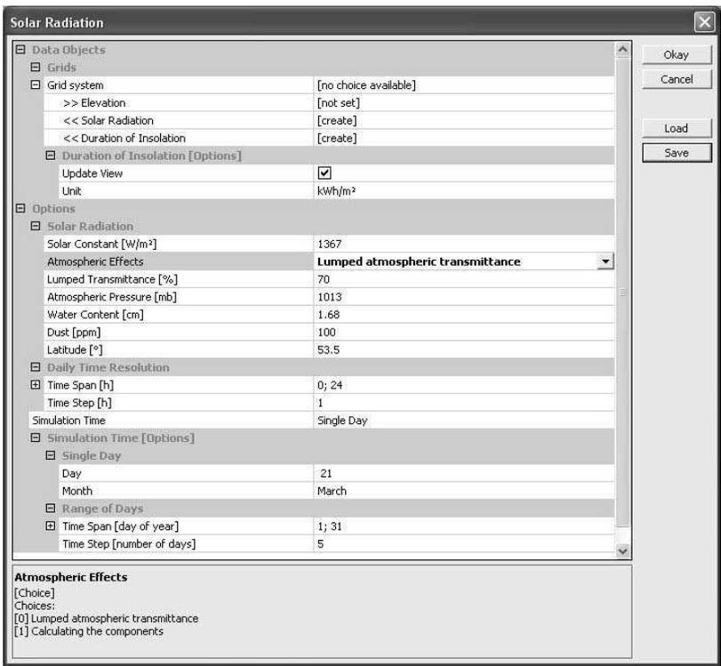
Figure 10.3. Solar radiation module interface in SAGA GIS software
