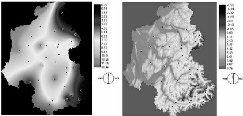
**Figure 8.1.** *Interpolation of the average temperatures in June for the Savoy and High Savoy departments. On the left, using kriging; on the right, using a linear altitude gradient*
