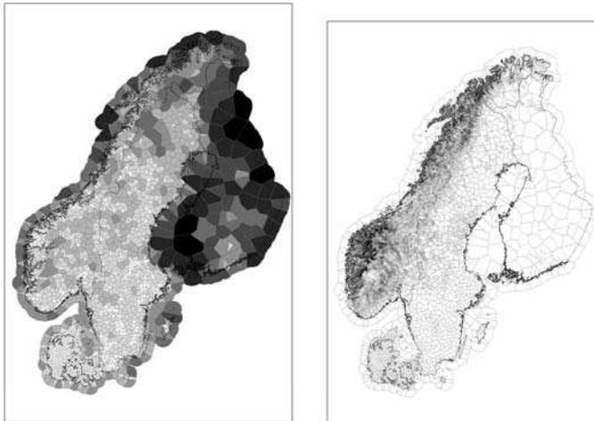
**Figure 6.1.** The left panel shows the (area of) Thiessen polygons of the meteorological network used for the NORDGRID project. The right panel shows the standard deviation of the terrain model (dark color for high standard deviation, light color for low standard deviation) indicating the variability of the terrain. Ideally areas with high variability should have higher station density
