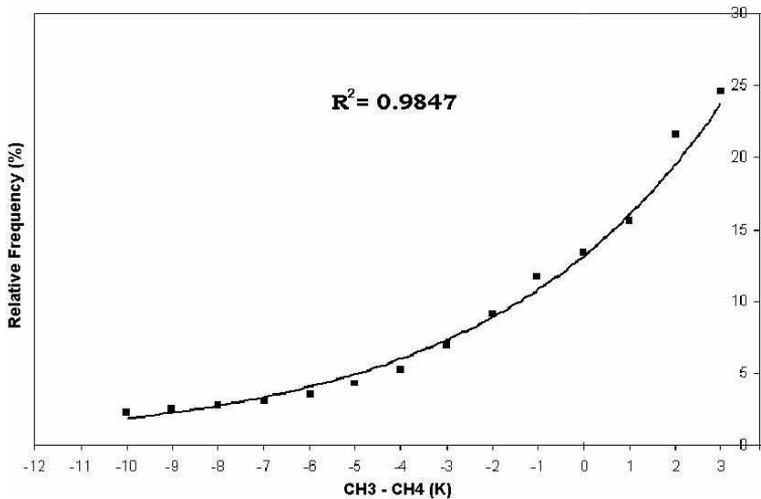
**Figure 2.3.** Probability of lightning occurrence. The values shown in the graph represent the frequency of lightning observed on the surface during two consecutive GOES-12 images as a function of the difference of brightness temperature between channel 3 and channel 4
