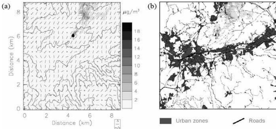
**Figure 20.8.** (a) Toluene concentration field in the finer-resolved domain (Domain 5) at 0900 UTC (1100 LT) on 17 August 2002. (b) Same results integrated into ArcGIS<sup>TM</sup> and superimposed on a layer representing urban zones
