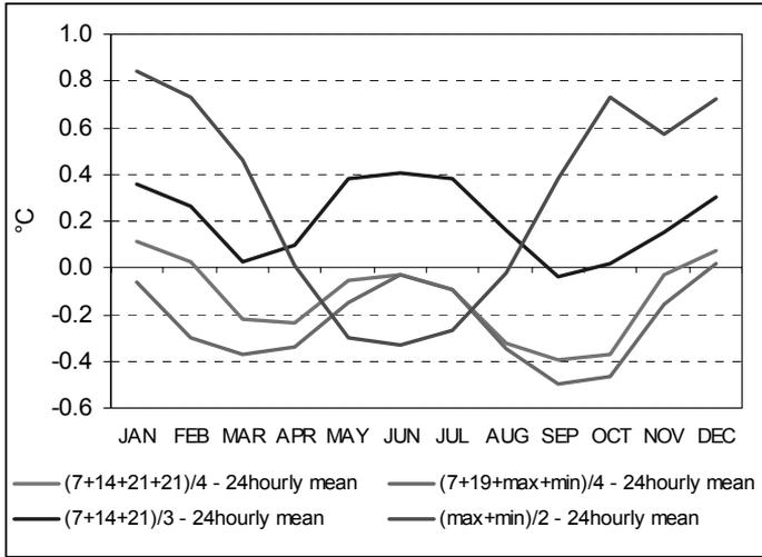
**Figure 15.2.** Comparison of the mean monthly temperature obtained by using different algorithms to calculate the monthly mean at the Austrian station of Puchberg. All values are shown as differences from the “true” (24 hours) mean
