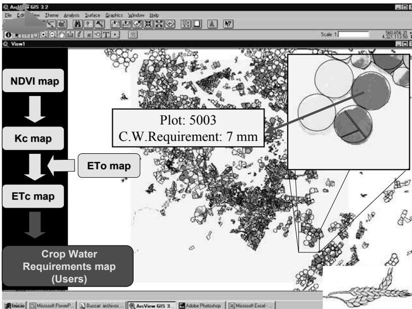
Figure 19.2. Diagram for crop water requirements derived from the EO data source
