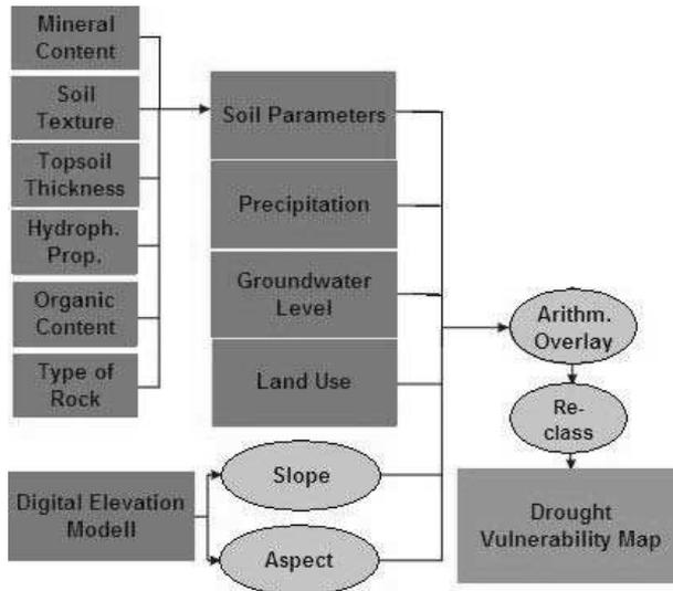
Figure 14.3. Flowchart of determination of drought vulnerability
