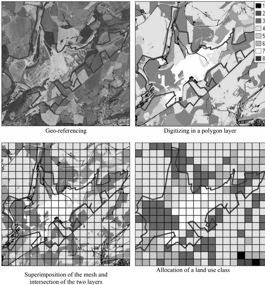
**Figure 20.6.** Necessary steps to assign land use to the finer grid (Domain 5)
