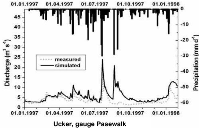
Figure 11.6. Daily rates of precipitation and simulated and observed discharge in 1997
