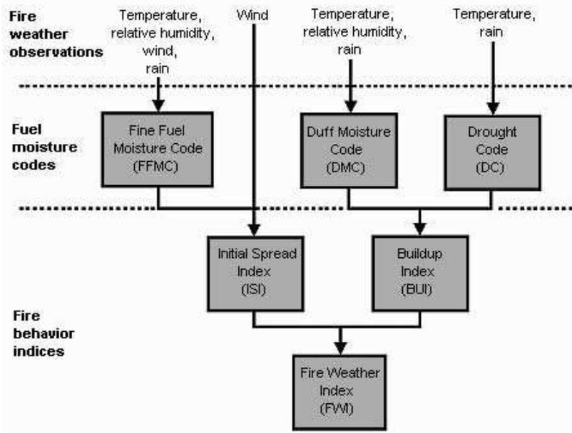
Figure 12.1. Fire weather index components [CFS 06]
