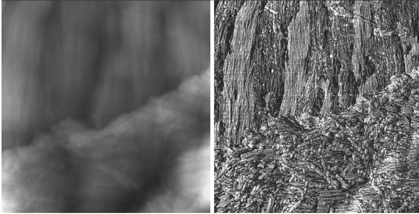
**Figure 3.2** Topography (left) and phase (right) images of an unbleached PGW fiber surface. The image size was  $3\ \mu\text{m} \times 3\ \mu\text{m}$  [7]. Instruments and settings: NanoScope IIIa Multimode scanning probe microscope, commercial Si cantilevers (Digital Instruments, Inc. Santa Barbara), tapping mode in air, resonance frequency 300–360 Hz, free amplitude  $\sim 20\ \text{nm}$ , set-point ratio  $r_{\text{sp}}$  0.4–0.6, no image processing.
