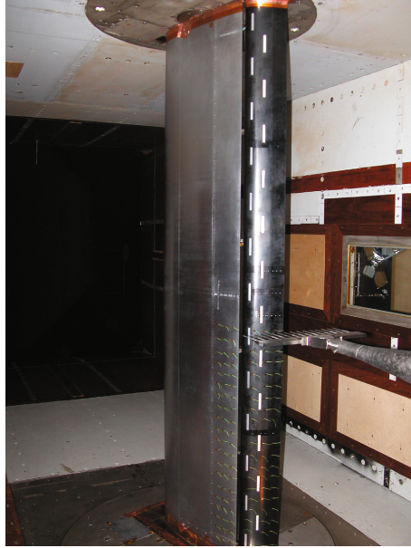
Fig. 5. DLR-F15 model mounted wall-to-wall in DNW-KKK cryogenic low speed tunnel
