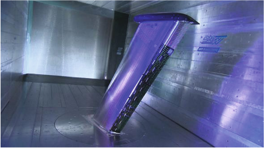
Fig. 7. DLR-F15 model mounted as 30°-swept cantilever wing in DNW-NWB atmospheric low speed tunnel
