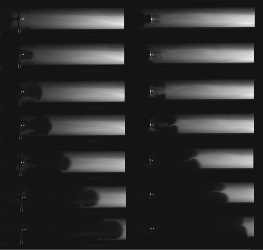
Fig. 7. High-speed images of accelerating flames using a single obstacle (Orifice A, left; Plate A, right), both having blockage ratios of 0.43. Time between two frames is 3\ \mu\text{s} .
