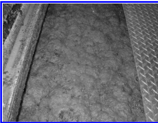
FIGURE 6.11 Excessive foaming in the first aeration tank in serially connected CSTR-based MBR, where the volume of the first aeration tank takes 1/7 of the total system volume.
