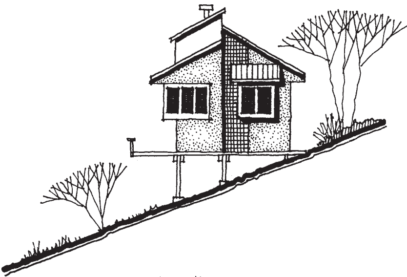
Post & beam construction
