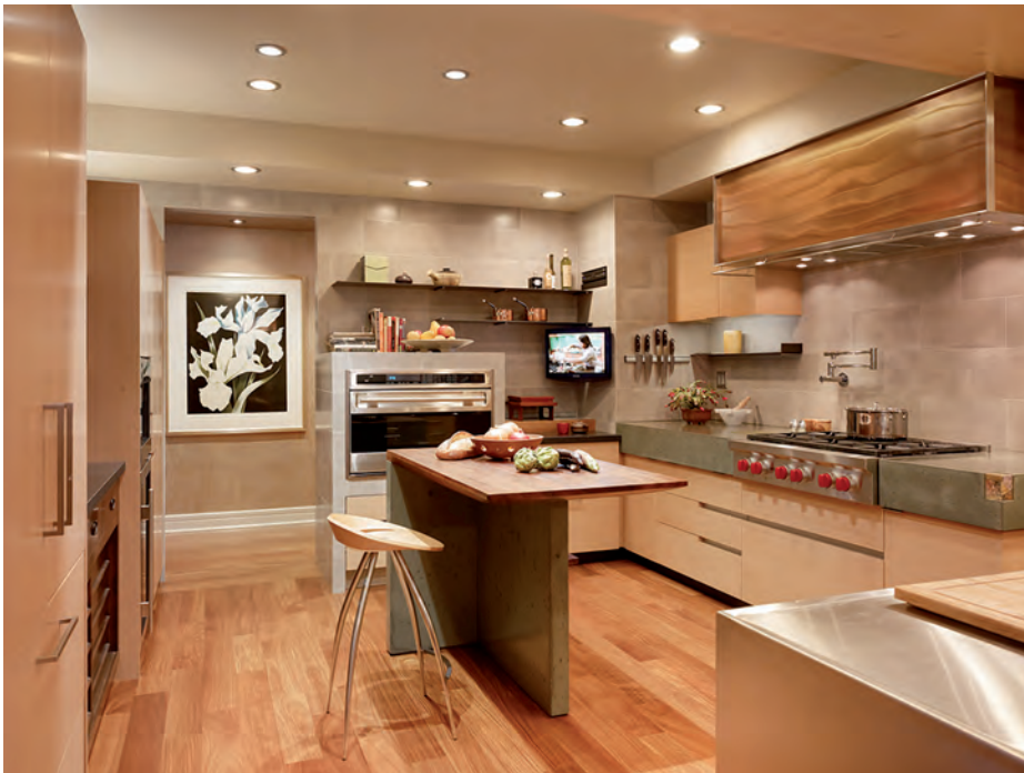
FIGURE 7.26 A kitchen with a concrete countertop. Concrete is used along the oversized backwall counter surface, as well as a support for the island.
