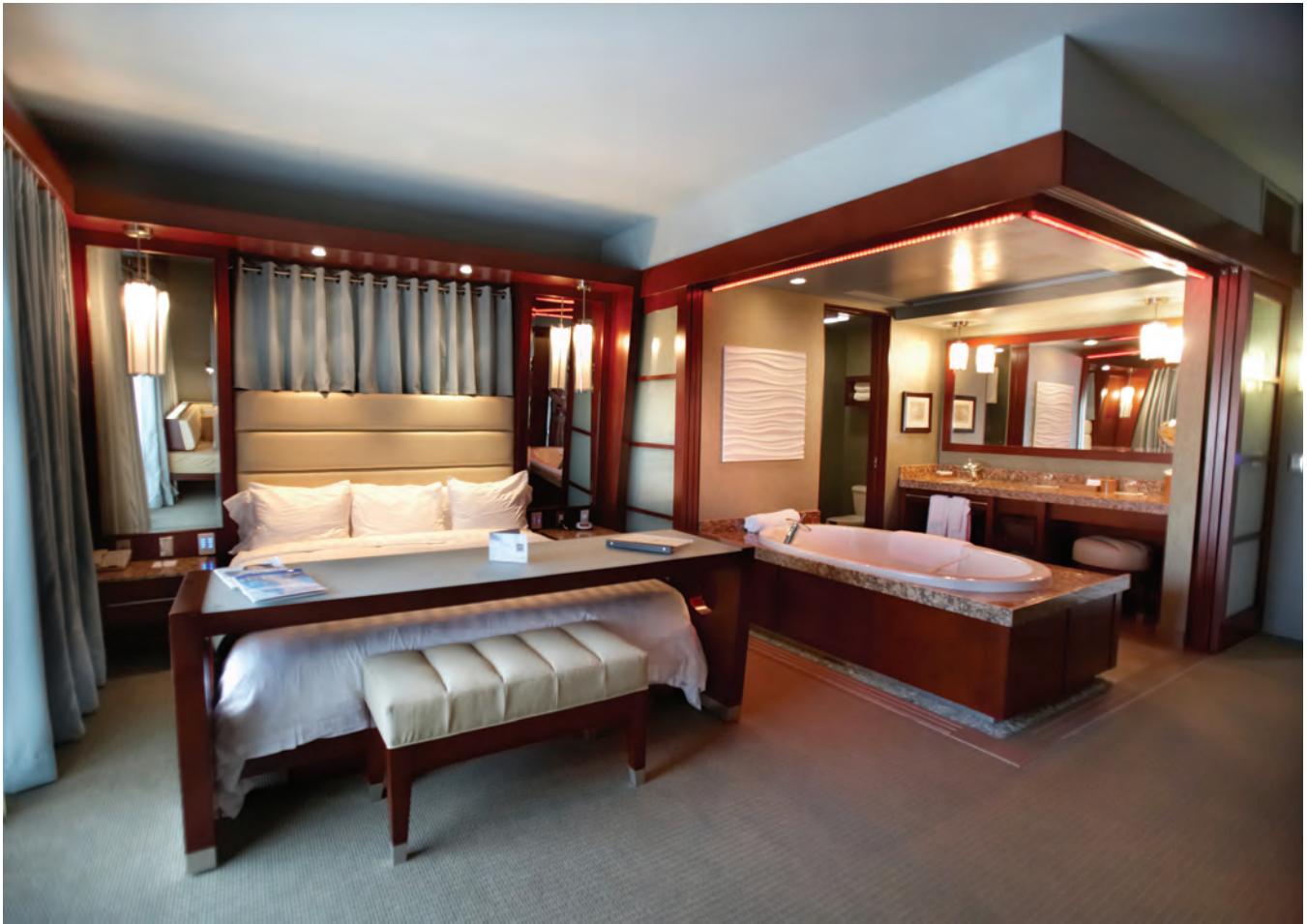
FIGURE 4.20 A platform bathtub can be top-mounted or under-mounted. In this example, it is top-mounted. In this design, a movable wall opens the bathing center up to the bedroom zone. The space is a hotel room at the Shade Hotel in Manhattan Beach, CA.
