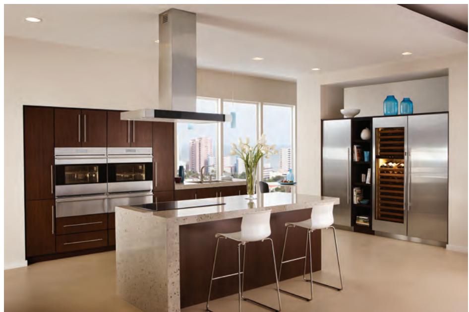
FIGURE 2.18 Single ovens can be installed next to one another for easy access. Note the placement of warming drawers below the ovens, making these appliances accessible as well.
