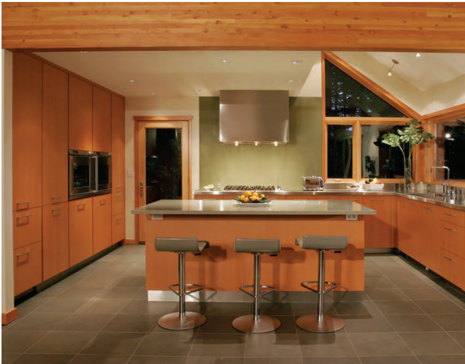
FIGURE 7.31 A kitchen combines a stainless steel countertop, a quartz island top, and a back-painted glass backsplash in the cooking area. Design by Martha Kerr, CMKBD
