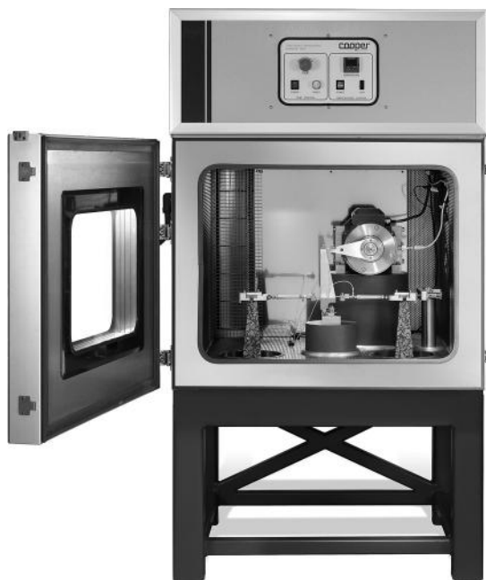
Figure 7.5 A two-point bending device on trapezoidal specimens. (Courtesy of Cooper Research Technology Ltd.)
