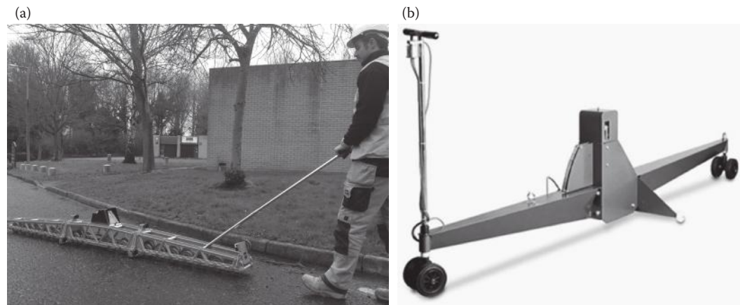
Figure 16.25 Rolling beam devices. (a) Rolling straightedge. (Courtesy of T&J Farnell Ltd.) (b) Travelling beam device. (Courtesy of Controls Srl.)
