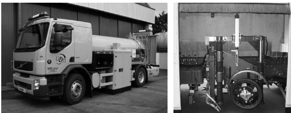
Figure 16.8 SCRIM and test wheel assembly (wheel in raised position). (Courtesy of WDM Limited.)
