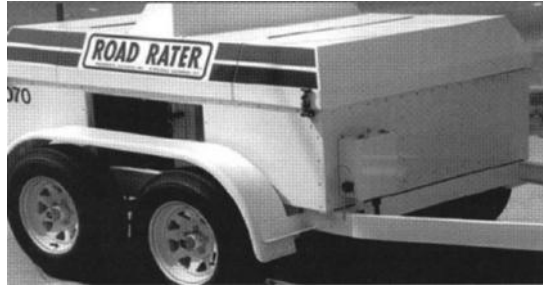
Figure 16.44 The Road Rater device. (From Asphalt Institute 3rd Edition, Asphalt Overlays for Highway and Street Rehabilitation . Manual Series No. 17 [MS-17]. Lexington, US: Asphalt Institute. With permission.)
