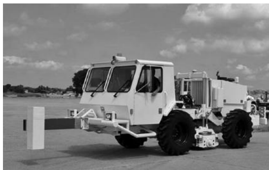
Figure 16.52 TPAD rolling dynamic deflectometer. (From Texas A&M Transportation Institute [TTI], Using New Technologies to Solve Old Problems , Texas Transportation Researcher, Vol. 49, No. 4, http://www.tti.tamu.edu , 2003.)
