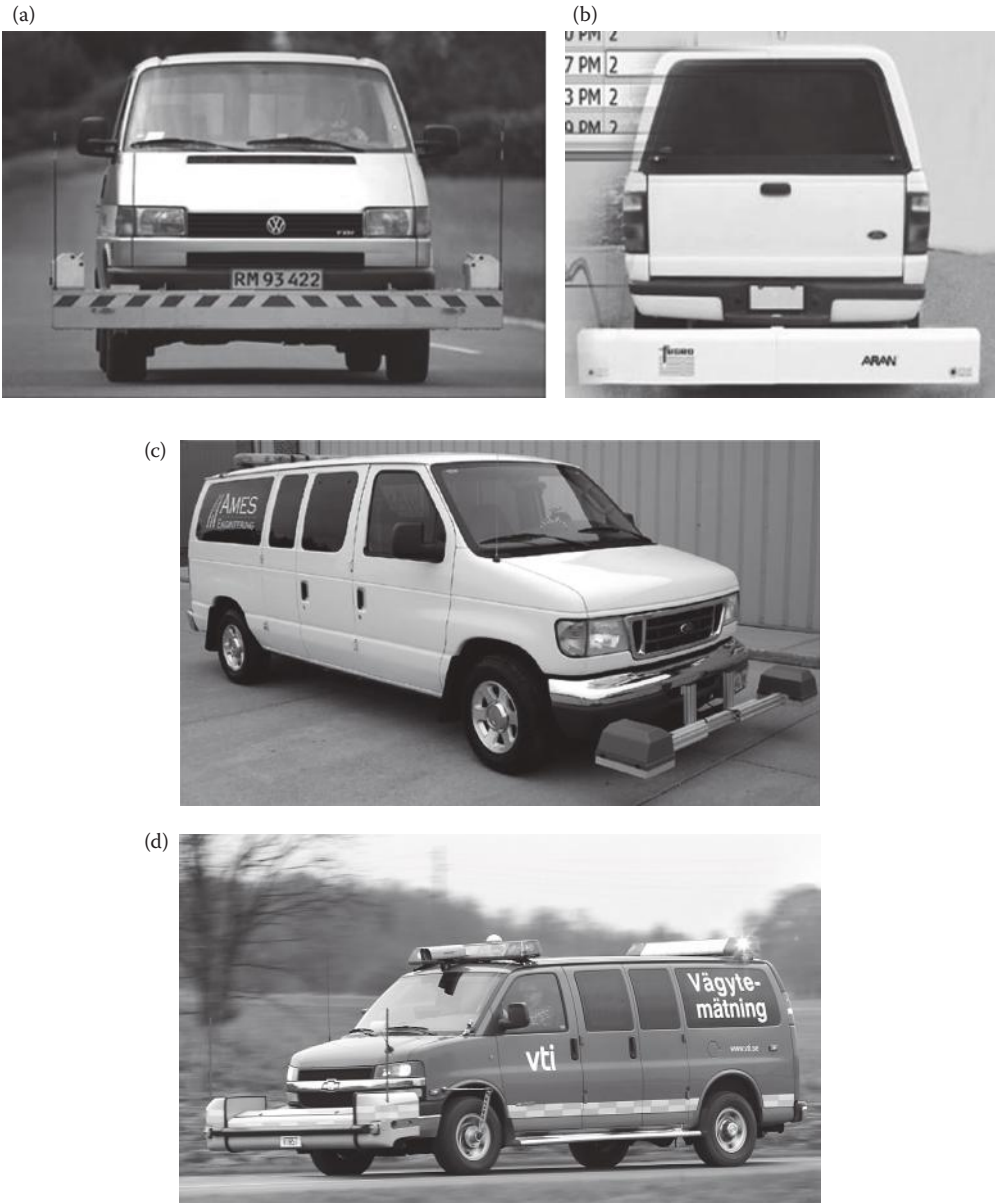
Figure 16.30 Some RSPs. (a) Dynatest RST-II (Dynatest International A/S). (b) Furgo ARAN 7000 (Furgo Roadware). (c) Ames 8200 high profiler (Ames Engineering Inc.). (d) VTI laser RST (VTI/Hejdlösa bilder AB). (Photos courtesy of the abovementioned companies.)
