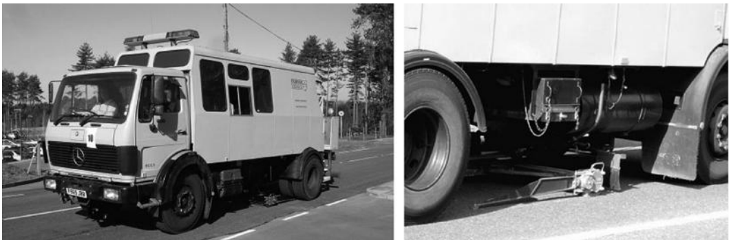
Figure 16.50 WDM Limited deflectograph. (From Highways Agency, Design Manual for Roads and Bridges [DMRB], Volume 7: Pavement Design and Maintenance, Section 3, Part 2, HD 29/08 , London: Department for Transport, Highways Agency, 2008b [© Highways Agency].)
