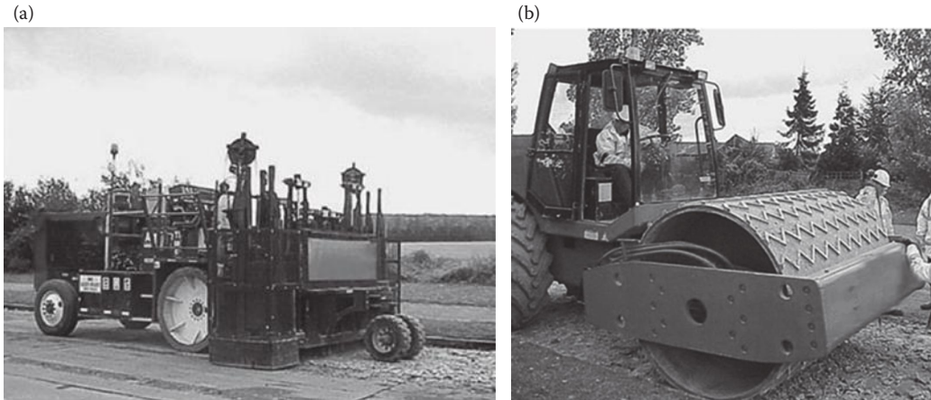
Figure 15.33 Equipment for rubblisation. (a) Multiple head breaker and (b) grid roller. (From Coley, C. and Carswell, I., Improved Design of Overlay Treatments to Concrete Pavements. Final Report on the Monitoring of Trials and Schemes . TRL Report TRL 657. Crowthorne, UK: Transport Research Laboratory, 2006.)
