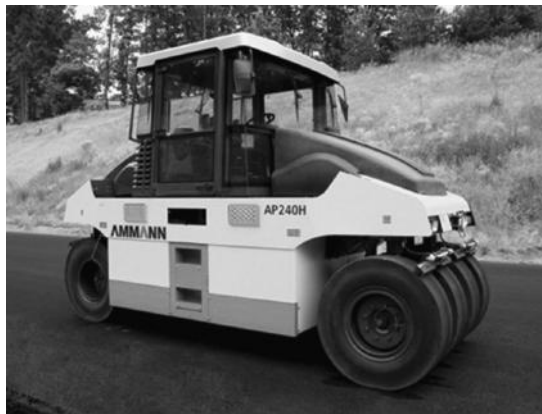
Figure 8.18 Pneumatic-tyre roller (four front and three back tyres). (Courtesy of AMMANN Group.)
