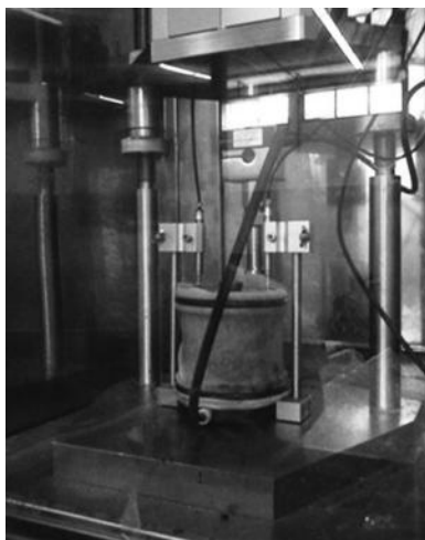
Figure 7.20 Triaxial cyclic compression test device making use of a partial vacuum as confining pressure.
