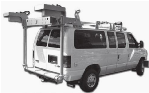
Figure 16.36 Pavement surface distress survey vehicles based on 3D laser imaging technology. (a) 3D laser image system and digital highway data vehicle. (Courtesy of WayLink Systems Co.) (b) Multi-functional vehicle (MFV). (Courtesy of Dynatest.) (c) ICC's 3D profiler. (Courtesy of International Cybernetics Corp.)
