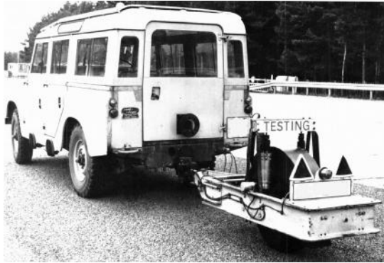
Figure 16.26 TRRL bump integrator on a trailer. (From Jordan, P.G. and Young, J.C., Developments in the Calibration and Use of the Bump-Integrator for Ride Assessment . TRRL Supplementary Report, SR 604. Crowthorne, Berkshire, UK: Transport Research Laboratory, 1980.)
