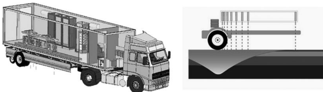
Figure 16.54 Second-generation TSD vehicle and deflection bowl. (From Krarup, J., Traffic Speed Deflectometer [TSD] . Measuring systems for infrastructure – For roads and for railroads, Sacramento, CA: FWD User's Group, 2012.)
