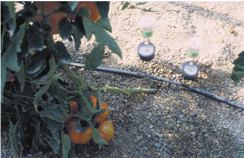
Photo 11.1. Tensiometers are increasingly used in greenhouses.
