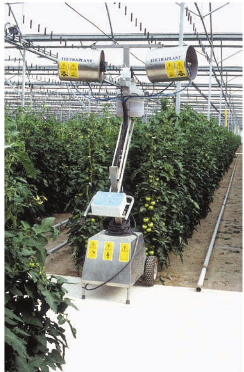
Photo 12.2. Mobile equipment for greenhouse pesticide treatments.
