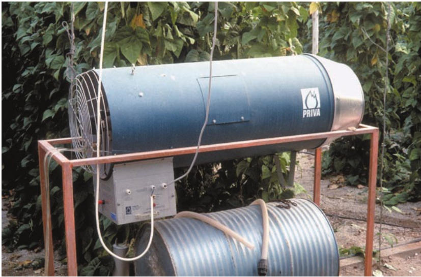
Photo 9.2. CO 2 generator that produces CO 2 by combustion.
