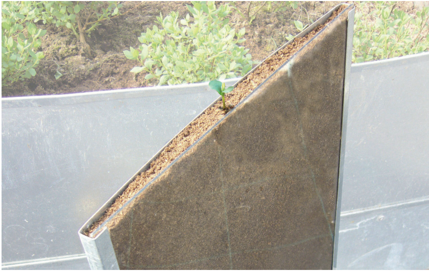
Fig. 7. The root box constructed from a metal frame and glass front wall used for the analytical assessment of the root growth and structures (Drobná, 2010).
