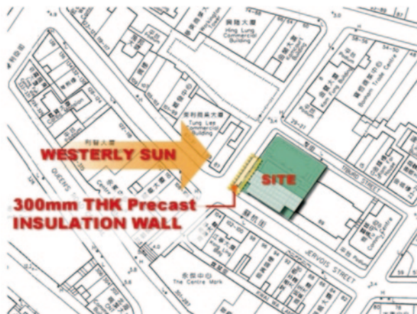
Fig. 7.3 Significant solar load from the west
