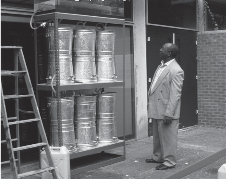
Fig. 12.6 Prof. Wole Soboyejo inspecting the modular water filtration unit prototype, used for testing flow rates and yields.
