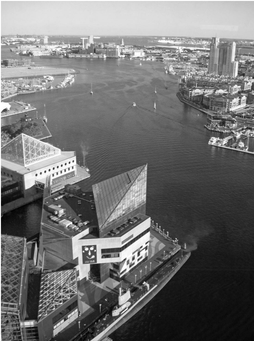
Figure 10-5. Entrance to the Baltimore Inner Harbor. The flow of tidal waters at flood and ebb are constricted as they flow into the Inner Harbor by a sea wall at Fort McHenry on the left and docks and bulkheads of Lazaretto Point on the right.
