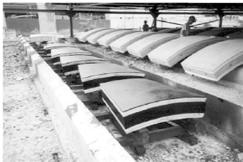
Figure 5 Precast segments following application of coal-tar epoxy resin coating
