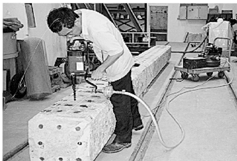
Figure 3 Typical pile being sampled for water-soluble chloride
