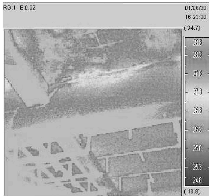
Figure 3 Infrared thermal images of a fire-damaged concrete building
