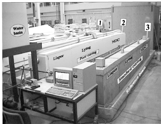
Figure 2 Overview of experimental set-up for large-scale chloride penetration test
