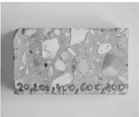
Figure 4 Digital photograph of the Penly concrete specimens exposed to 1 hour at 200, 400, 600 and 800 0 C
