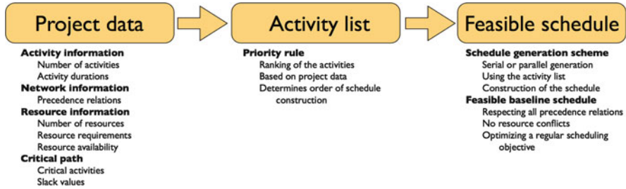
Fig. 5.16 The priority rule based scheduling approach to construct a feasible project schedule
