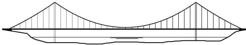
(a) Suspension bridge
