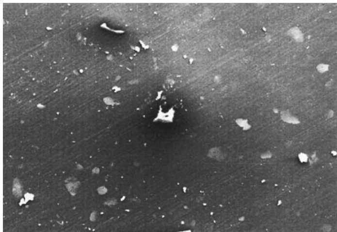
Figure 37 Scanning electron micrograph of metal flake paint for trucks showing entrained dirt and intentionally added metal flakes. The particulate material in this micrograph averages several micrometers in diameter.
