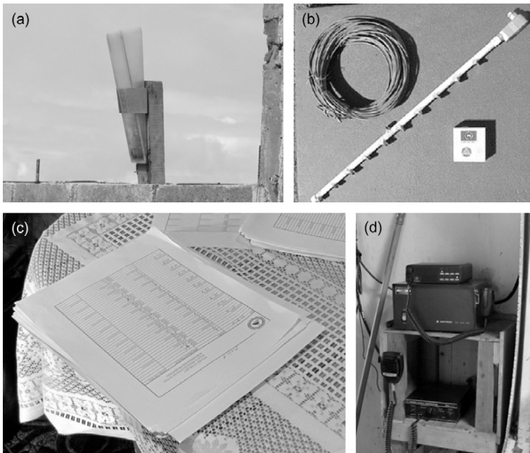
Fig. 5. Image of the Equipments and Material Used for the RELSAT. (a) Plastic Pluviometer; (b) Equipment to Gauge River Water Level Installed in the Upper Area; (c) Data Sheet to Record the Daily Precipitation; (d) Radio Communication Equipment. Source: Photo by CNE.
