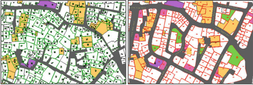
Fig. 4.13 Plot reorganization seen at neighborhood level (shaded plots are those where buildings survived the quake and blank ones where buildings collapsed) (EPC and GUDC 2002)
