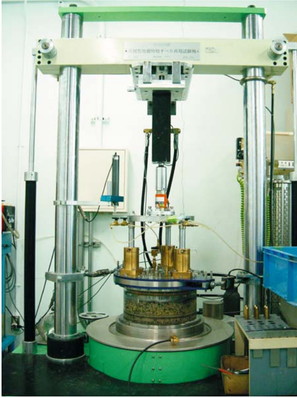
Fig. 18.2. Overview of the ring shear apparatus with a transparent shear box (DPRI Ver. 7)
