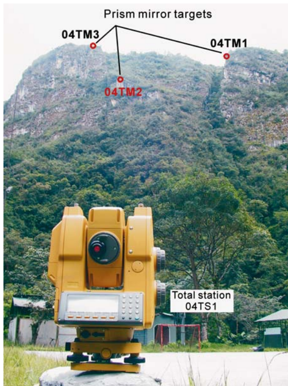
Fig. 2.14. Total station and location of prism mirror targets placed on the head of toe cliff of the block no. 2
