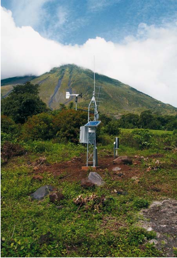
Fig. 41.7. Meteorological station installed in the Concepcion Volcano in Nicaragua, forming a part of a pilot landslide early warning system
