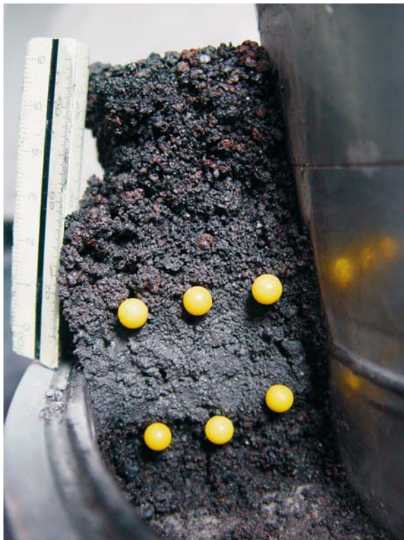
Fig. 21.8. View of the shear zone after the test
