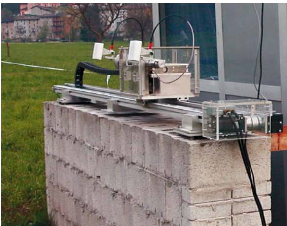
Fig. 43.3. Picture of the LiSA system installed in front of the Cortenova rock slide. The radar rail was placed on a concrete wall specifically built for the monitoring
