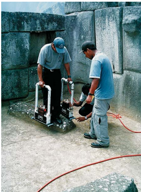
Fig. 5.2. This figure shows the sensors and software 200 MHz transmitter and receiver antenna assemblies. Not shown is the Pulse-EKKO 100 console and the recording laptop computer
