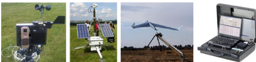
Fig. 4 Basic ESS equipment (from left): meteorological sensors with INCA modem, unmanned ground station (UGS), unmanned aerial vehicle (UAV), IMSI catcher
