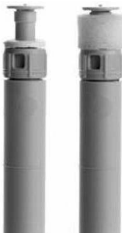
Fig. 3. Collection device before (left) and after (right) completion of the sampling process.
