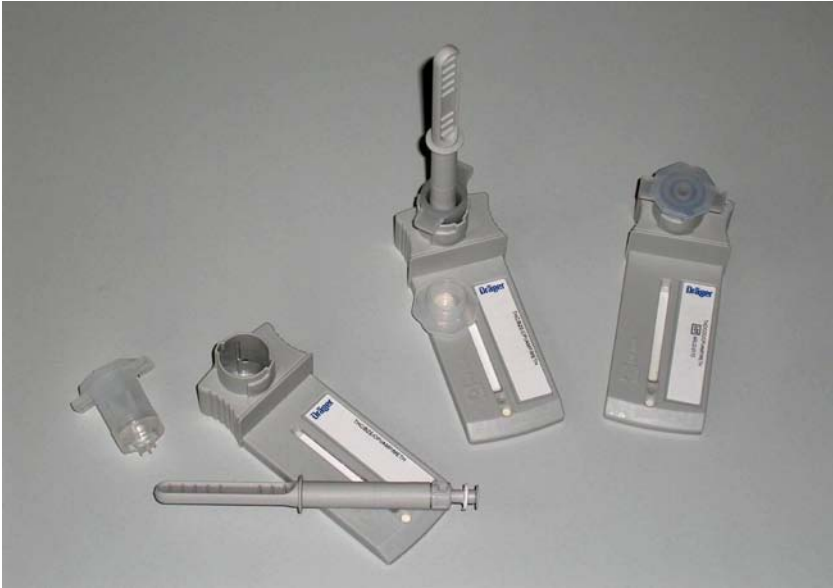
Fig. 1. Dräger DrugTest® Kit for oral fluid samples (collection device, test cassette and inserted sample preparation cartridge).
