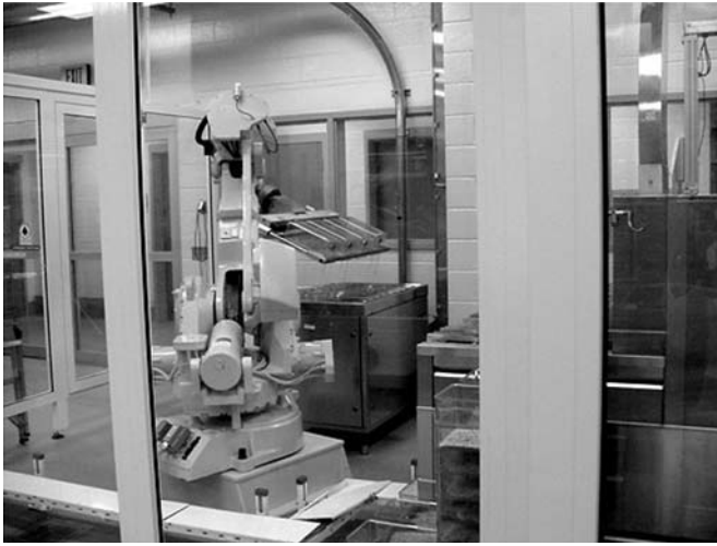
Fig. 12-8 Robotic cage-washing system showing both the soiled-side robot (left) and clean-side counterpart (right). The soiled side also shows the dirty bedding dumping station (D), in conveyor track (I) and first tunnel washer section (T). On the clean side are bedding cages on the out conveyor (O), automated bedding dispenser (B) and egress section of the tunnel washer (T).
