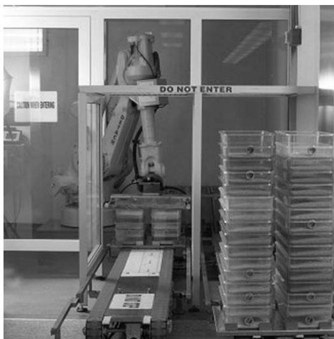
Fig. 31-16 Robotic cage cleaning. Clean side robot filling sanitized rodent boxes with bedding and placing them on a conveyor.
