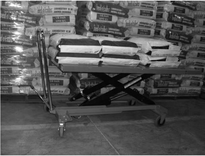
Fig. 12-4 Adjustable (scissors) dunnage rack allows for the loading and unloading surface to be adjusted as needed to the safe height for any worker.
