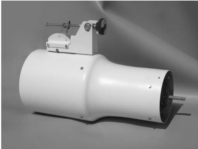
Fig. 20-18 A venturi-type PICV. The knob on the top of the device is used to adjust the volume of air provided by the device within its design specifications.
