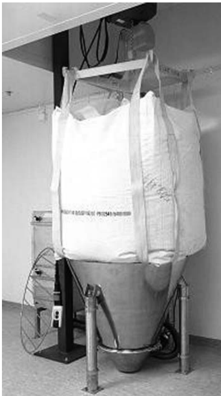
Fig. 12-5 Overhead emptying of a bulk bag of contact bedding into a bedding system load funnel enabled by a hoist and rail overhead system.
