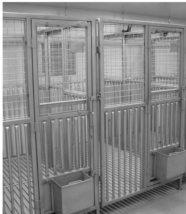
Fig. 22-2 Stainless-steel runs constructed of a combination of tubular materials and mesh on the upper panels with raised fiberglass slat flooring panels. The runs are 4' × 6' in dimension with sliding gates between the runs allowing for pair- or group-housing of adjacent animals as needed. The room is configured for wet sanitation with a trench drain and flush mechanisms (not visible) located behind the runs and a central ceiling-mounted hose reel.
