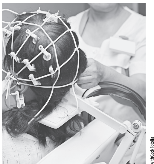
FIGURE 9.1 Illustration of subject wearing the geodesic sensor net of 64 electrodes.
