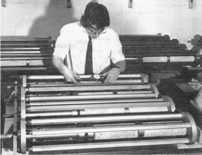
**Figure 16.18** Measuring strain of concrete specimens with a 200 mm demountable mechanical Demec strain gauge.
