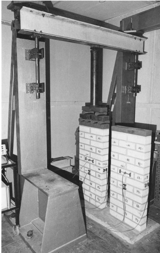
**Figure 16.2** Double lever arm system for applying a sustained load to a calcium silicate wall located behind a load-free control wall [7].
