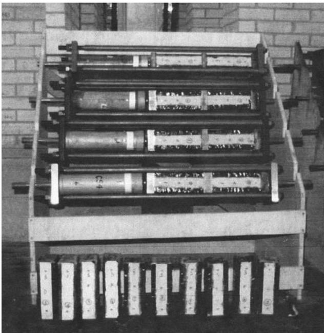
**Figure 16.6** Part-sealed mortar prisms under load for determining creep and corresponding control prisms for determining shrinkage. Part sealing simulates volume/surface ratios of mortar in different types of brickwork indicated in Figure 16.7 [19].
