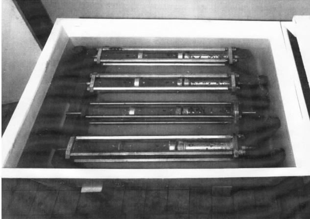
**Figure 16.8** Load test frames stored in water to measure basic creep of concrete; control specimens also stored to measure swelling.
